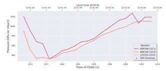
The same analysis performed on temperature was used for the pressure readings. As the rocket reached peak height, pressure levels fell. Once the CanSat got separated from the rocket and started its descent, the pressure started to rise again.
