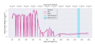
Our mission was to collect environmental parameters like Particulate Matter and CO2 levels. The latter was not collected due to programming errors. The Particulate Matter sensor, being connected to UART, worked well, and we have data readings from our mission. In the graph, the level of PM particles dropped as the CanSat rose. There are a few spikes in the data, but we think they might have been created by air movement caused by the rocket itself.
