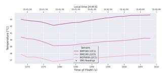
We analyzed the core mission phase when the rocket rose and then came down with the CanSat. From the graph, one can see that the ascension to the peak point took 10 seconds and the descent took 38 seconds. Even so, temperature readings were performed during landing, but the number of records is not impressive.
