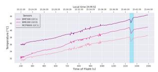
The temperature was measured using three sensors: the Bosch BMP388, the Bosch BME280, and a Microchip MCP9808. The sensors were all placed in different places and experienced different conditions during the flight. Since there are many "extra" temperature differences in the graph, those could be caused by the different airflow channels and different proximity to heating sources such as the OBC.
