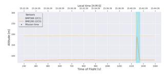
Altitude was recorded using sensors on two I2C buses. Because we had average-to-low signal quality, we had readings from only one of the two GPS modules. As for pressure, because Altitude is inversely related to Pressure, the graph presents a pretty sharp rise in altitude once the launcher rose toward the top altitude spot and a similar drop back to the airport's ground altitude.
