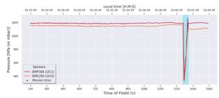
The pressure sensor data was gathered from two simultaneous I2C buses with two Bosch sensors BMP388, BME280. One can see on the graph that the pressure from both sensors drops once the rocket lifts off and then spikes when the CapSt time caught.
